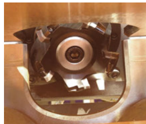
High-speed rotary milling head with replaceable carbide Inserts
