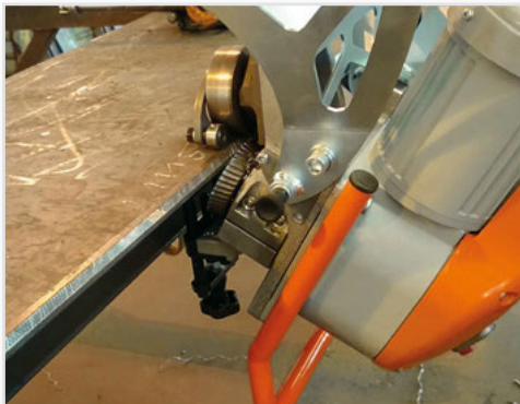
Adaptor for beveling pipe & round tubes 3-3/4" and larger
